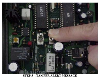
Next, press the right switch down (while the left switch is in the up position) to *replay* the tamper alert message. The recording is now complete. If you would like to re-record your message, repeat STEP 2.
