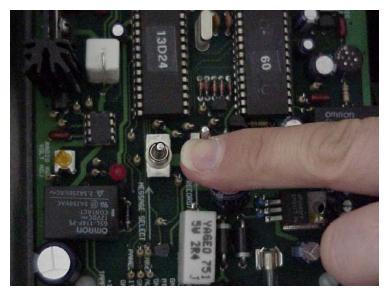
**STEP 5 – ID/LOCATION MESSAGE** Next, press the right switch up (while the left switch is in the center position) to *record* the call box ID/location message.
