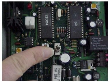
STEP 1 – TAMPER ALERT MESSAGE Position the left switch up to select the Tamper Alert Message. Sample Message – "Tamper Alert, Tamper Alert"
