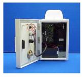
Check that the microphone and wiring harness are still connected to the circuit board as shown below.
