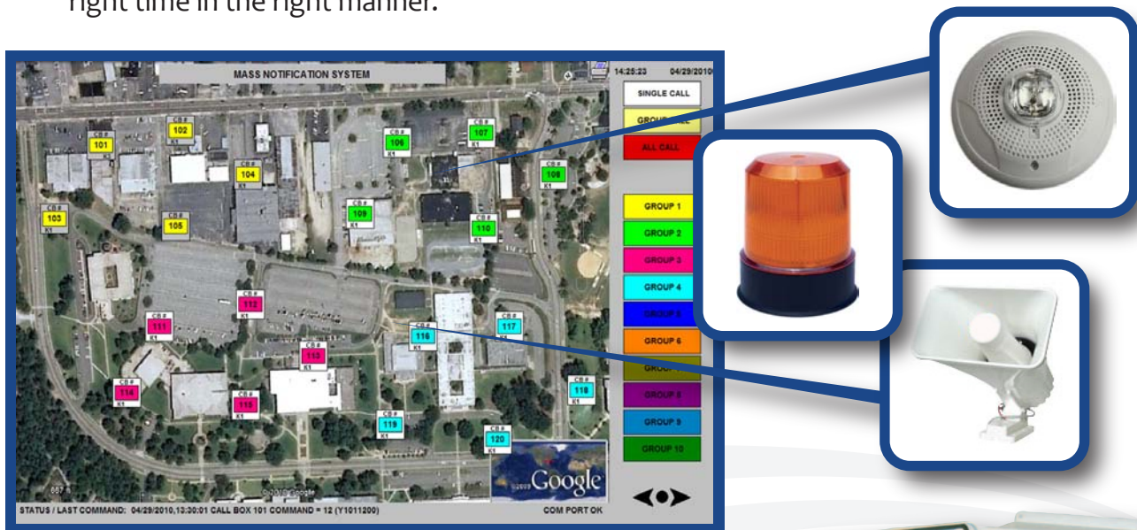
Shown (clockwise): Mass Notification System Map, Strobe Light Unit, Indoor Speaker/Strobe, High Power Outdoor Speaker
